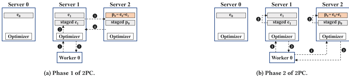
Figure 4: Toy example of the 2PC protocol used in ECRec with k = 2 and r = 1 .
